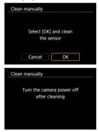
3. Remove the lens and clean the sensor.
